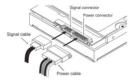
Figure 4. Attaching SATA cabling
